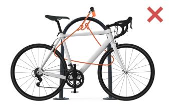
The Approved D-Lock is attached to the Immovable Object only and not through the main frame, with only the non-approved Accessory cable securing the Bicycle.
