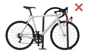
The lock immobilises the front wheel, but it doesn't pass through the main frame of the Bicycle and the Bicycle stand. The main frame of the Bicycle must always be secured to an Immovable Object with an Approved Lock.
